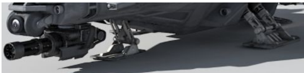
7.9.1 - articulated landing skids and rotatable nose-cannon
